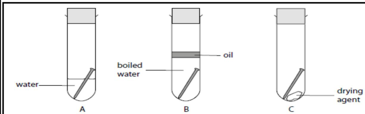
In the diagram, only the nail in test tube **A** will rust. This is because it is exposed to both **oxygen** and **water**.
