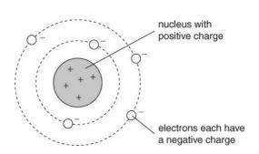
A positively charged object will attract a negatively charged object. Two objects with the same charge (both positive or both negative) will repel each other.
