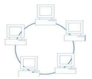
In a ring network, computer systems are connected in a ring or a loop. Around the ring, packets are sent, being passed from one computer system to the next until they arrive at their destination.
