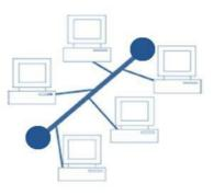
The computer systems, also called *nodes* of the network, are each connected to a single cable on which data can be sent, called the bus. A bus network has terminators on each end, which is needed to ensure that the network functions correctly.
