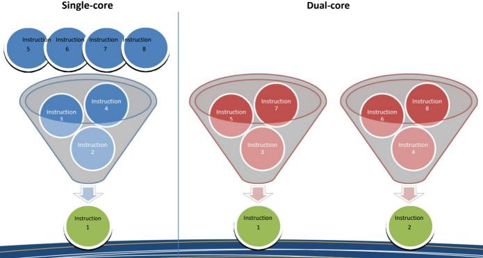
In a single-core CPU each instruction is processed one after the other, whereas in a dual-core CPU, two instructions may be processed at the same time. In theory, a dual-core CPU should be able to process instructions twice as fast as a single-core CPU. However, this isn't always the case as sometimes *Instruction 2* may need the result of *Instruction 1* before it can be processed.
