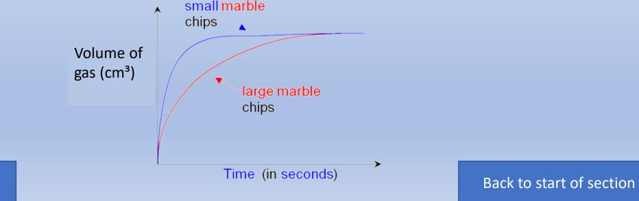
The graph for the small pieces of marble chips is steeper- larger surface area- faster rate of reaction (steeper the gradient)
